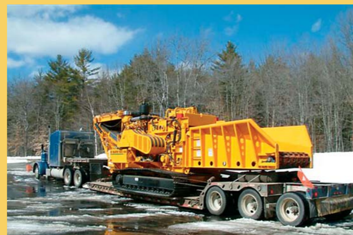
At only 78,000 pounds, the 6800 is specifically engineered to be transported on a standard lowboy.
